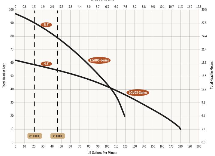
Pumps must operate within the proper range shown on the performance chart. It is the responsibility of the end user to ensure this requirement is met. Pumps operating outside the recommended range are prone to damage, excessive vibration, cavitation, poor efficiency, and may exceed nameplate amperage.
